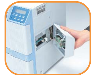
Optional in-line contactless smart card encoding module
